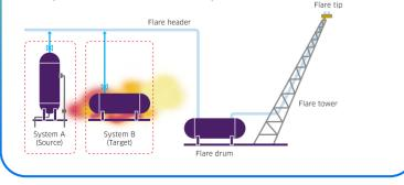
In collaboration with our Health Safety and Environment Design department and the Process and Technologies division, we provide a performancebased flare system design to define the optimized depressurization flow rate in line with material selection for equipment design, survivability of equipment from fire impact and personnel evacuation time.
