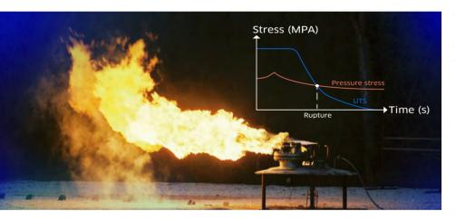
We use in-house software LNGDYN® for dynamic depressurization calculation, considering equipment rupture aspect through DYNSURV®. Our approach is based on the fundamental process safety rules.
